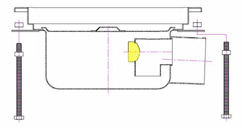
\* IN CASE APPLICATION OF ADJUSTING FEET IS REQUIRED, AS A FIRST STEP, THE BOLTS AND NUTS ARE FIXED ON THE BODY AS SHOWN BELOW.
