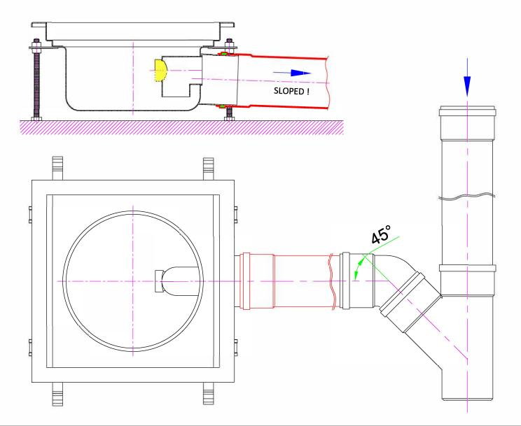
\* APPROXIMATELY 30-40 MM OF CONCRETE IS POURED AT THE BOTTOM OF EACH FOOT AND LEFT TO CURE. MAKE SURE THAT THE FLOOR DRAIN IS KEPT UNTOUCHED TILL THE CONCRETE IS PROPERLY CURED.
