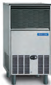
B 7040 Ice production & storage @ 10°C Air-10°C Water 75 Kg/24h @ 21°C Air-15°C Water 71 Kg/24h Bin storage 40 Kg Dimensions WxDxH: 54 cm x 60 cm x 103 cm*
