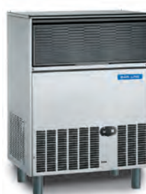
B 8040 Ice production & storage @ 10°C Air-10°C Water 88 Kg/24h @ 21°C Air-15°C Water 82 Kg/24h Bin storage 40 Kg Dimensions WxDxH: 70 cm x 60 cm x 102 cm*
