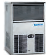
B 2615 Ice production & storage @ 10°C Air-10°C Water 28 Kg/24h @ 21°C Air-15°C Water 26 Kg/24h Bin storage 15 Kg Dimensions WxDxH: 47 cm x 57cm x 69 cm*
